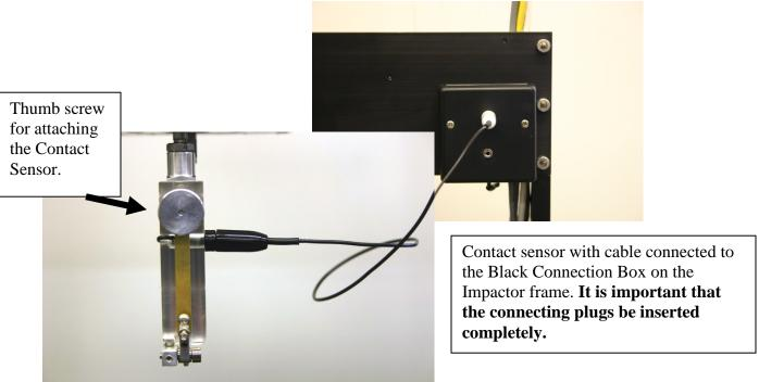
• It is very important that the head of the Impactor tip and mounted Contact Sensor do not rotate during this procedure
