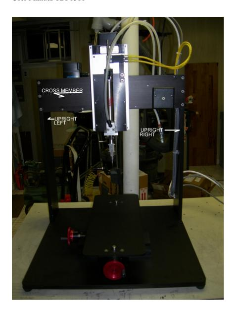
Set the base down. The uprights will be vertical with the offset step facing the front.
